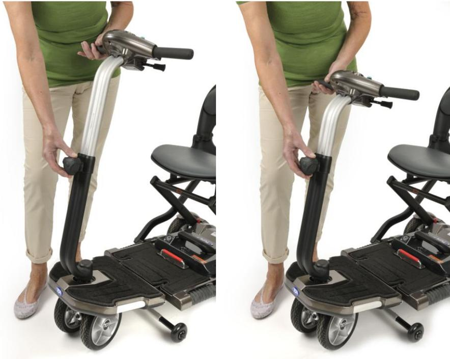
If you'd like to adjust the height of your Minimo tiller simply turn the adjustment wheel anti clockwise until the top part of the tiller moves freely up and down. Then just move the top half of the tiller to the height you would like and tighten the adjustment wheel by turning it clockwise until tight.
