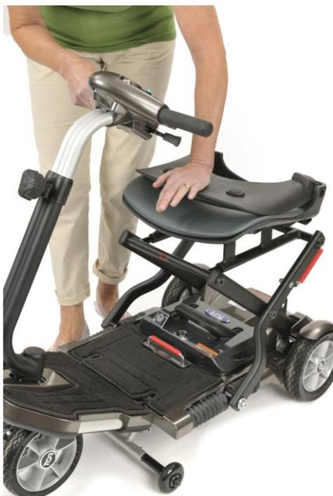
3. Use one hand to push the seat down towards the floor pan and the other to move the tiller towards the seat which will lift the front wheels off the floor and fold your Minimo.
