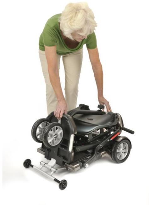
Once folded you can then lift your Minimo using the handle at the rear and stand it on its front wheels to move around in the folded position.
