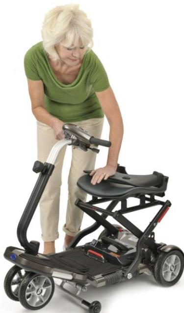
4. Finally push the tiller against the seat and the front of the floor pan towards the rear wheels to ensure your Minimo is locked into the folded position.
