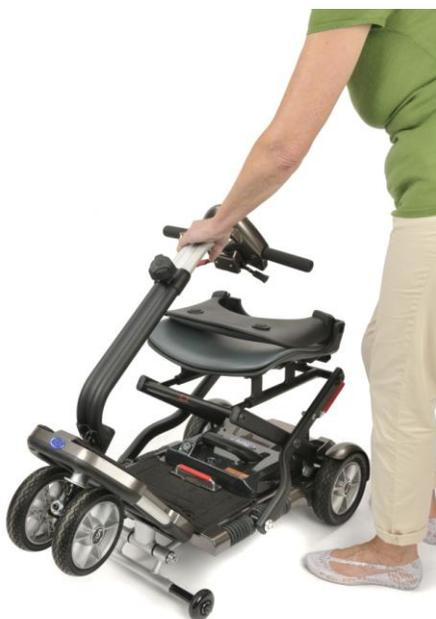
3. Ensure your Minimo is locked in the unfolded position by pulling the chair away from the floor pan with one hand and pushing the tiller away from the seat with the other until you hear a click and feel you Minimo lock into this position. Once your Minimo is locked in position you will no longer be able to move the tiller towards and away from the seat so use this as a simple test to find out if you Minimo is locked in the unfolded position.
