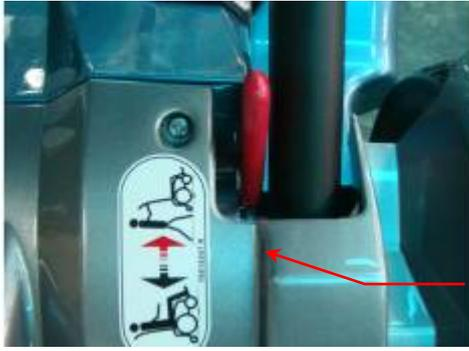
Free- Wheeling Lever/ Maximum required hand-arm force on the lever is 19 N for engaging and 35 N for disengaging
